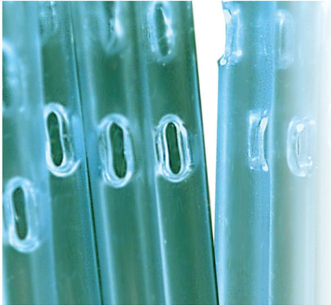
PlasticWeld's HPS05-DB 2-up polished eye former was originally developed for the urinary drainage catheter market, where smooth-edged eyes are a critical performance feature. A proprietary actuator system provides precise control of the eyelet-forming punches, and is adaptable from 5 Fr up to 22Fr tube sizes.
