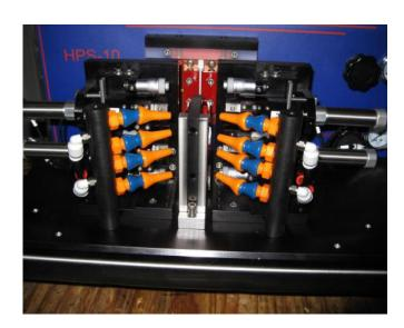
PlasticWeld's HPS05-DB 2-up polished eye former was originally developed for the urinary drainage catheter market, where smooth-edged eyes are a critical performance feature. A proprietary actuator system provides precise control of the eyelet-forming punches, and is adaptable from 5 Fr up to 22Fr tube sizes.
